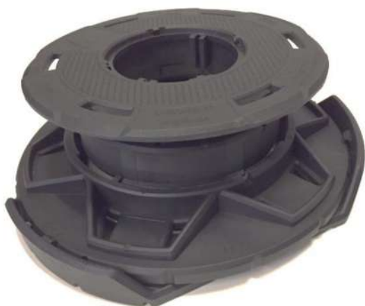
Figure 3: Sample 3 - Lower column raised, upper column collapsed, screw retracted
